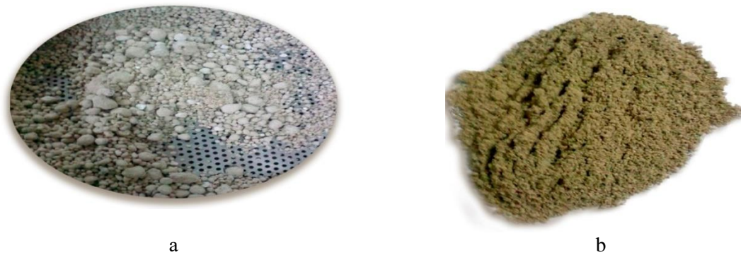
Figure 2. Appearance of phosphogypsum: a – phosphogypsum from the first sample (apatite concentrates from the Kola Peninsula); b – phosphogypsum from the second sample (phosphorite concretions from the African continent).
