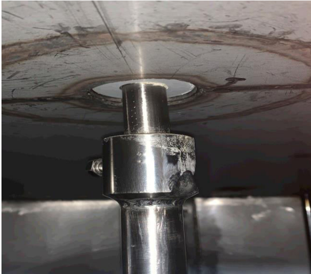
Figure-2. The unit of friction and sealing of the cantilever shaft of a mechanical mixer with an installed experimental sleeve made of PCM based on fluoropolymer and silica gel.
