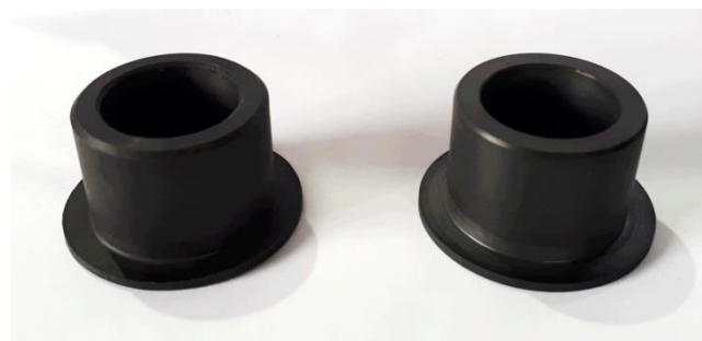
Figure-4. Bushings of the sliding bearings of the sections of the John Deere 1780 sowing complex of the "mushroom" type from the developed polymer material based on aromatic polyamide.
