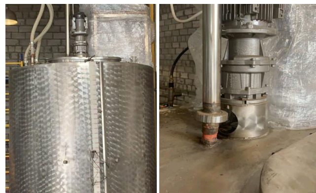
Figure-1. General view of the anchor stirrer (a) and friction and sealing unit of the anchor stirrer (b).
