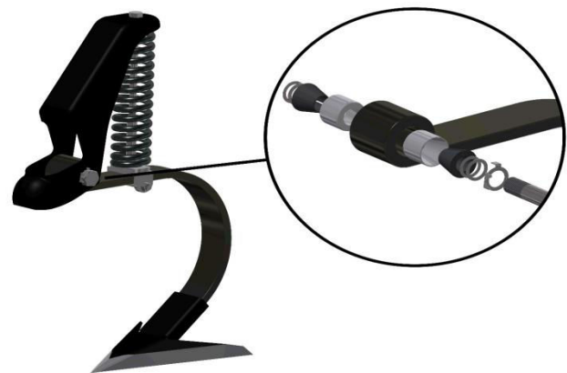
Figure-7. Cultivator paw arrow and bearing assembly with experimental design of damping mechanism assembly.
