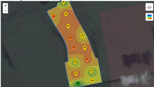
Fig. 9 – Results of soil hardness measurements of field T18.
