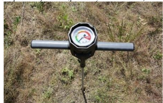
Fig. 2 – Penetrometer of mechanical type. No GPS tethering.
