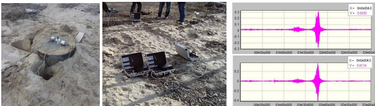
Figure 1. Equipment for vibration monitoring and an example of vibration signals recorded as a subway train passed by.
