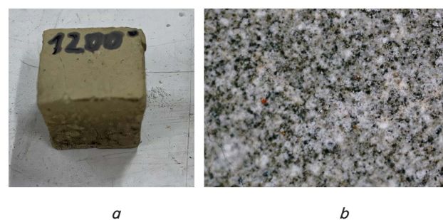
Fig. 7. The sample fired at a temperature of 1200 °C: a – photograph; b – photomicrograph
