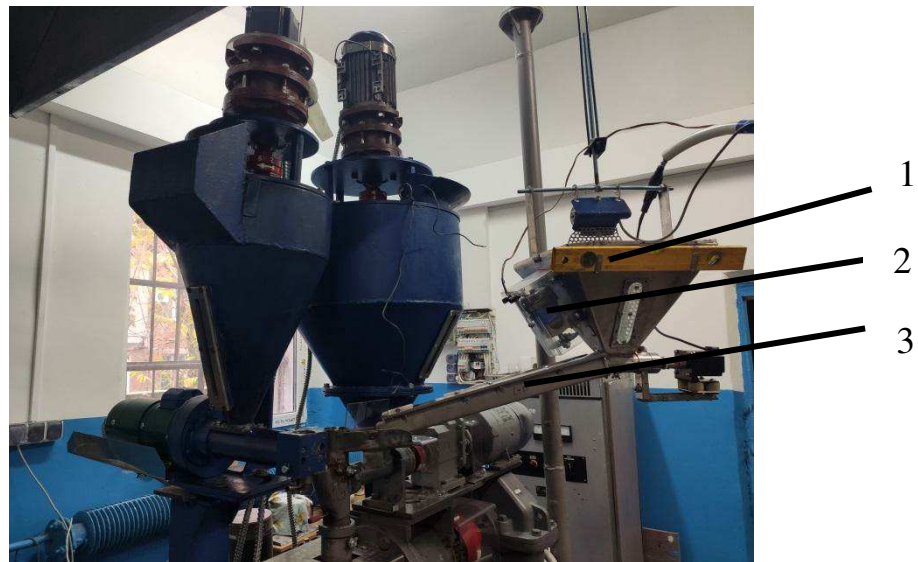
Fig. 1. Feeder system: 1 – hopper; 2 – vibration motor; 3 – tray
