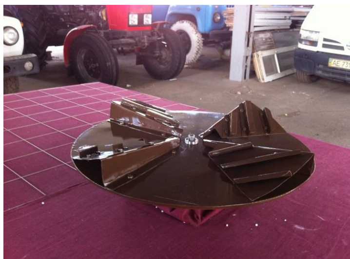
Fig. 2 - Upgraded centrifugal spreader disc
