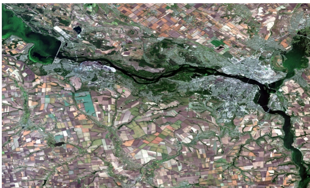
Fig. 4. Sentinel-2B/MSI multispectral satellite image over the Mokra Sura river area for 2017.09.19, 13 spectral bands, 10 m spatial resolution
