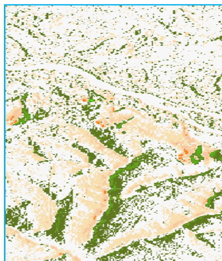
Fig. 1. Changes in terrain elevation in the basin of the Mokra Sura river by Sentinel-1A/InSAR data processing
