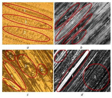
Fig. 9. Metallographic images of the working surfaces of the samples of polymeric and steel materials: a – reference sample of the polymeric material; b – examined polymeric material; c, f – steel samples, ×400
