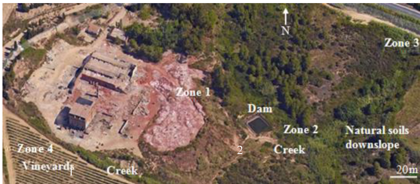
Fig. 1. View of the Demimesa area emplacement few months after the closure. Hazardous waste landfill and the surrounding affected natural and agricultural fields may be noticed. The surface has been divided into 4 zones to evaluate the impact of contamination by metal(oid)s.
