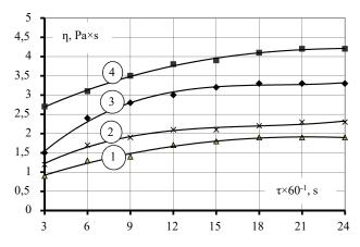
Fig. 1. The dynamics of effective viscosity of the additive solutions during hydration in the environment of cow's milk ( $t=20\pm2$  °C,  $\gamma=50$  s<sup>-1</sup>):
