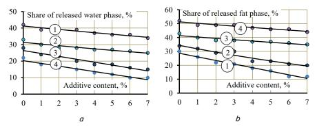
Fig. 4. Dependence of the emulsion stability on the content of the additive and different fat content after heat treatment (*t*=90...95 °C, τ=3×60 s): *a* - the share of the released water phase; *b* - the share of the fat phase released; 1 - proteinmineral additive; fat content, 40 %; 2 - protein-mineral additive; fat content, 60 %; 3 - improved protein-mineral additive; fat content, 40 %; 4 - improved protein-mineral additive; fat content, 60 %
