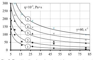
Fig. 7. The effective viscosity of emulsion samples based on butter with the addition of the improved proteinmineral additive at a temperature of  $20\pm2$  °C: 1 - control; 2 - 1 % additive; 3 - 3 % additive; 4 - 5 % additive; 5 - 7 % additive
