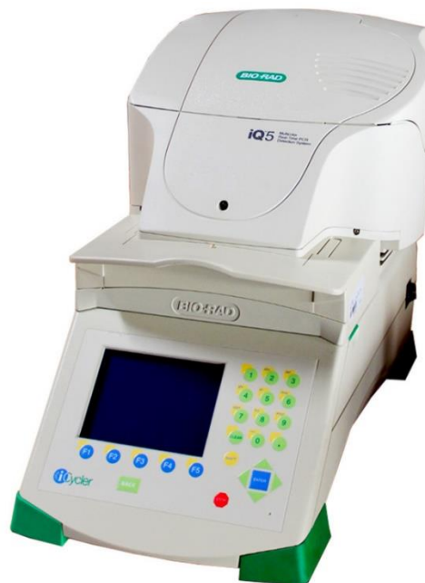
Рис. 71. Ампліфікатор Bio-Rad iCycler Thermal Cycler with iQ5 Multicolor Real-Time PCR Detection System
