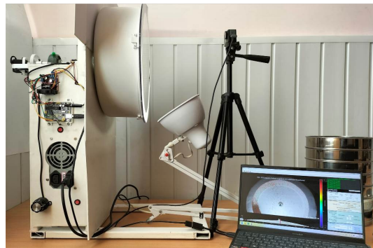
Fig. 21. Structural and technological scheme (a) and general view (b) of a laboratory cylindrical cell: 1 – bed frame; 2 – bearings; 3 – empty shaft; 4 – cylinder; 5 – glass cover; 6 – plates with cells; 7 – the pulley is known; 8 – drive pulley; 9 – solid shaft; 10 – direct current electric motor; 11 – Arduino UNO control board; 12 – L298N DC motor driver; 13 – potentiometer; 14 – power supply unit; 15 – tray; 16 – servo drive; 17 – video camera Aspiring Repeat 4 Ultra HD 4K Dual Screen ; 18 – IR sensor; 19 – cold white lighting lamp (5000–6500K)
