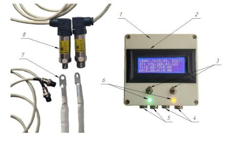
**Figure 2.** Appearance of the device for measuring the pressure and temperature of the working fluid: 1 – computing unit, 2 – display, 3 – toggle switches, 4 – temperature sensor ports, 5 – pressure sensor ports, 6 – workflow indicators, 7 – temperature sensors, 8 – pressure sensors
