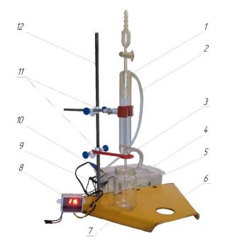
*Figure 1.* Installation for determining the kinematic viscosity of the oil at a given temperature: 1 – viscometer, 2 – feed tube, 3 – drain tube, 4 – water tank, 5 – pump, 6 – stand, 7 – working fluid sample tank, 8 – thermostat, 9 – temperature sensor, 10 – electric heater, 11 – viscometer holders, 12 – rod
