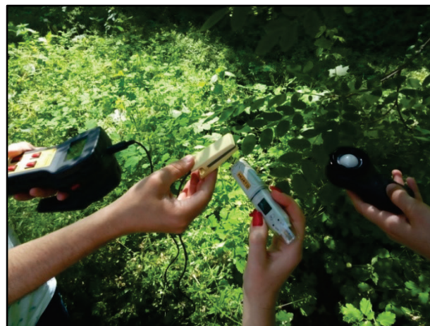
Fig. 1. Instrumental support of the experiment: Floratest, Thermo-hygrometer NE-173 and PCE-174 Lux Meter
