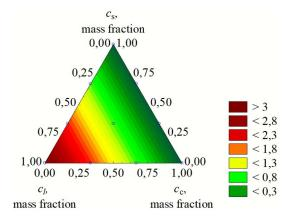
Fig. 1. Dependence of the ω-3:ω-6 PUFA ratio of the blend of unrefined first cold-pressedlinseed, corn and sesame oils on their ratio
