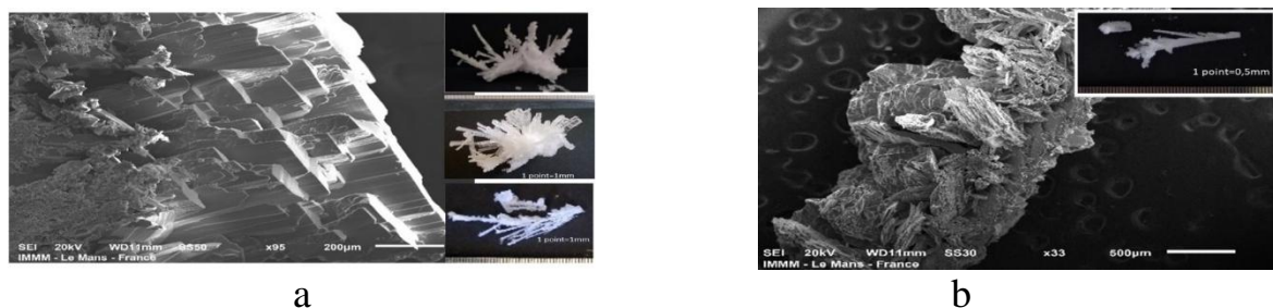
Fig. 14. Photomicrographs of gypsum crystals grown with the following additives to the crystal forming medium: a) – SiC nanoadditive (5%) and Sika superplasticizer; b) – SiC nanoadditive (10%) and Sika superplasticizer (0.2%)
