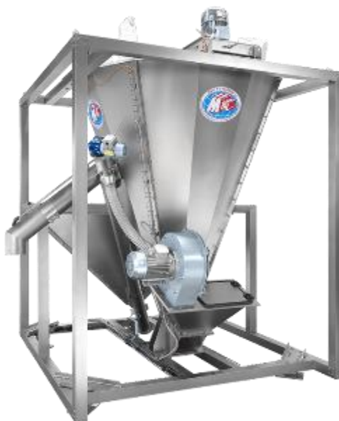
Рисунок 2.3 Compact Mill and Mixer for 1 ton/h Animal Feed Production Plant
