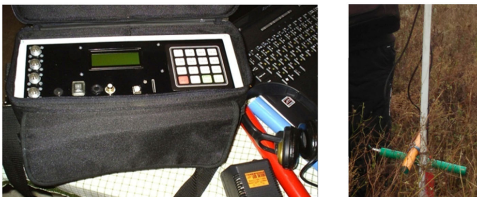
Figure 4. General view of the “SIMEIZ” device and antenna placement for NPEMFE signal detection.
