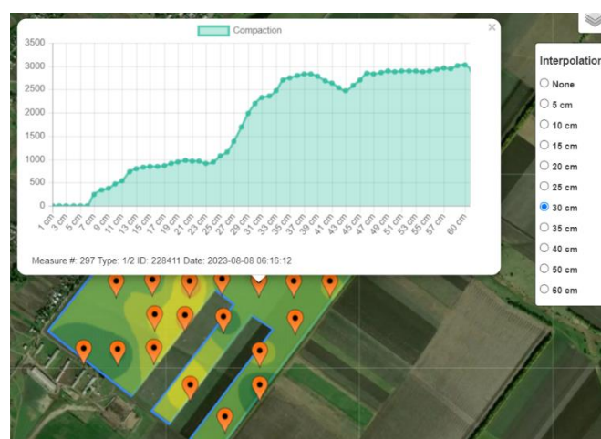
Fig. 1. Characteristic dependence of soil hardness on depth on experimental field No. 1.
