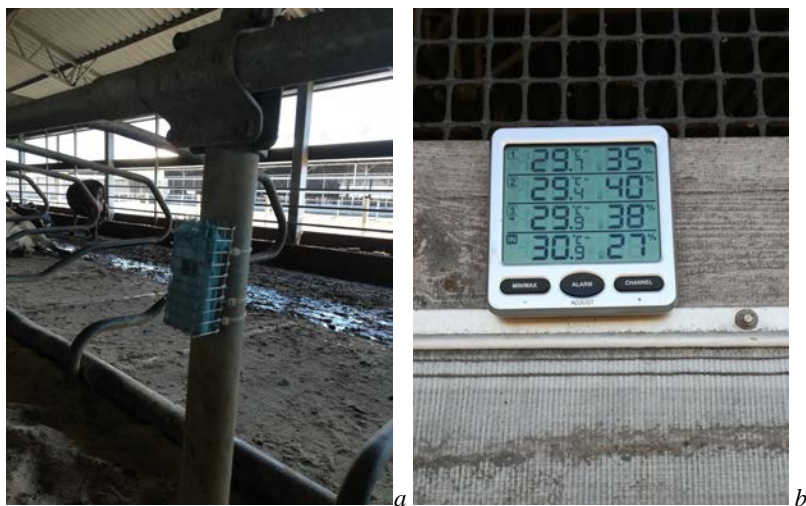
Figure 1. Measurement of temperature and humidity mode in one of the uninsulated barns: one of the sensors (F007TH) is located in the cow resting stall (a), the Ambient Weather WS-10 thermohygrometer is placed outside the barn (b)
