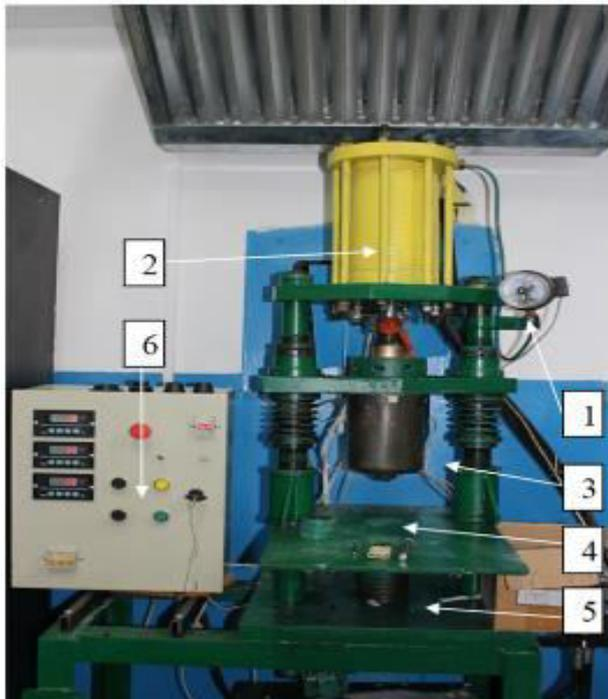
**Figure-2.** The casting press machine of manual type PL-32: 1- a pressure gauge; 2- hydraulic cylinder; 3- heating chamber; 4 - nozzle; 5 - the platform; 6 - control panel.
