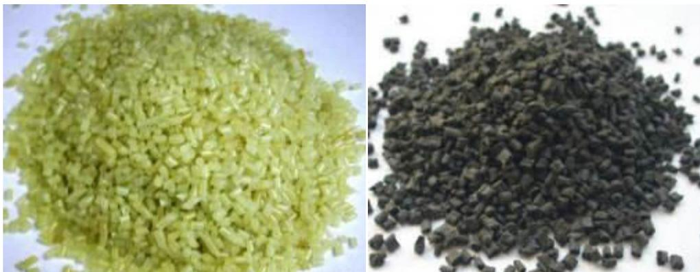
**Figure-3.** The main view of granules for recycling: Nylon 66 and UPA-6-30.
