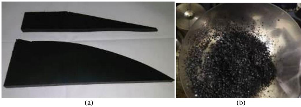
**Figure-4.** The main view of elements of used exhausted polyethylene PE-500 before (a) and after (b) comminuting.
